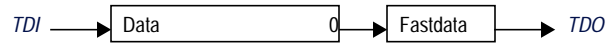
Figure 11.16 TDI to TDO Path When in Shift-DR State and FASTDATA Instruction is Selected
